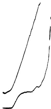
Fig. 4.—Effect of carbon dioxide on phytol wave of chlorophyll a. Lower curve: chlorophyll a alone. Upper curve: chlorophyll a and carbon dioxide. Sensitivity 50 of Sargent Polarograph. Camera opened at 1.60 volts applied cathodic potential. Diffusion current of lower curve: 3.4 microamperes. Approximate concentration of dioxane extract: 3.7 millimoles per liter.
